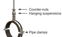
The hanging suspensions should be placed at the ends, i.e. at the top and bottom, if possible:
