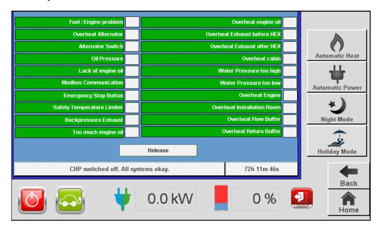
The system constantly monitors different temperatures and states. If certain limit values are exceeded here then a safety shutdown takes place automatically. Possible causes of a safety shutdown are displayed on this screen. The corresponding messages have a green background.
