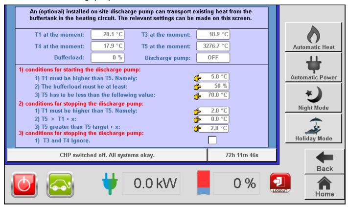
A discharge pump installed by the customer can pump available heat into the heating circuit. Trained specialist personnel are able to stipulate the behaviour of the system and the connected discharge pump in this menu.
