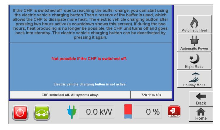
When the buffer tank is full, the system switches off.
