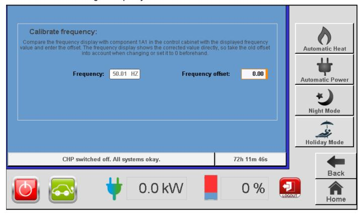
It is possible to enter and adjust an occurring deviation (offset) from the electricity meter to the screen value if necessary. The electricity meter and software calibrate to the same value.
