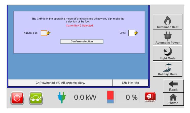
Menu for selecting the fuel - natural gas or LPG (liquid petroleum gas).
