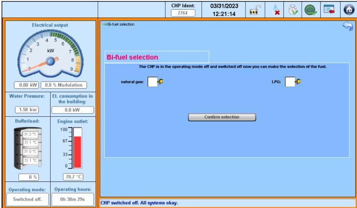
Menu for selecting the fuel - natural gas or LPG (liquid petroleum gas).
