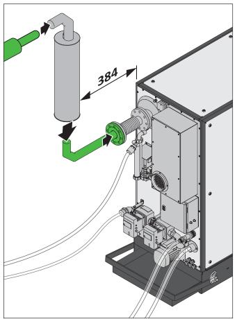
The line must be laid with a sufficient gradient to the generation unit.
