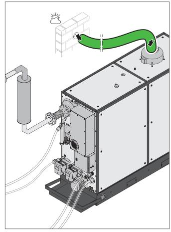
The line (e.g. flexible aluminium tube) must be flexibly connected and removable for maintenance work.
