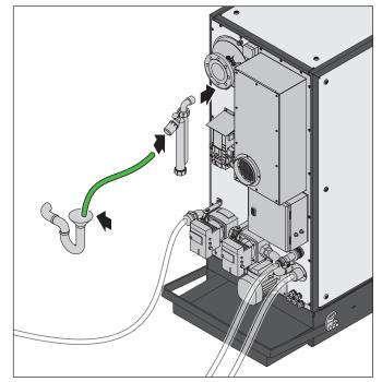
The line for the condensate water must be corrosion resistant.
