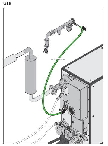
The gas supply must comply with the established regulations (e.g. in Germany, TRGI). Connection via a gas appliance outlet is not permitted.
