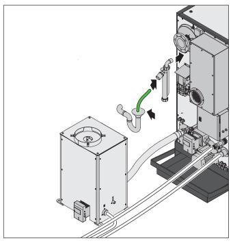
The line for the condensate water must be corrosion resistant. The line must have a sufficient gradient between the generation unit and the drain.
