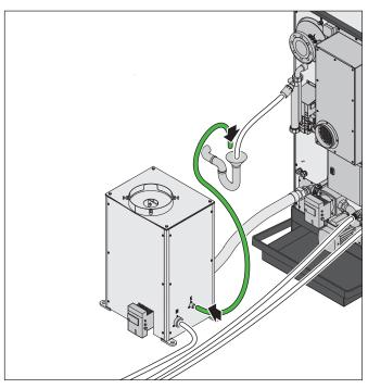
The line for the condensate water must be corrosion resistant. The line must have a sufficient gradient between the calorific value heat exchanger and the drain.
