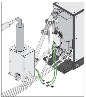
Connect the cable from the calorific value heat exchanger to the generation unit.
