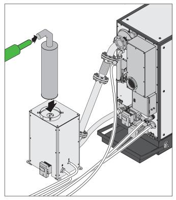
The line must be laid with a sufficient gradient to the calorific value heat exchanger.
