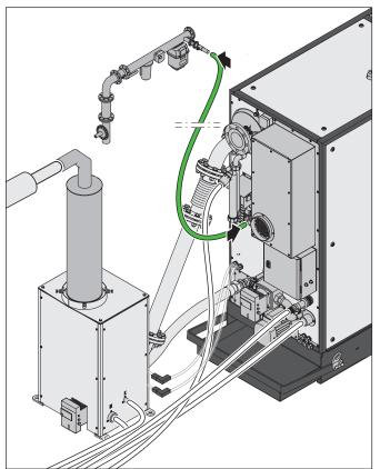
The gas supply must comply with the established regulations (e.g. in Germany, TRGI). Connection via a gas appliance outlet is not permitted.
